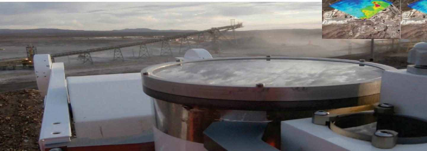
*Image of a Raymetrics LIDAR in use for dust pollution tracking in a mine in Chile*
